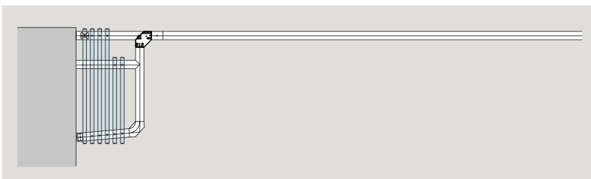
Stacking panels of varying width.
